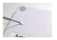
2.2 Use a coin to turn the battery door anti-clockwise; remove it from case.
