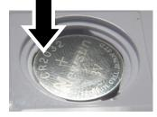
3.2 Replace the battery door; turn clockwise to lock it into place.
