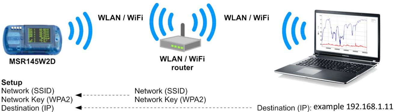
In this option you do not require any additional hardware, as it uses the existing network infrastructure. There is no Internet access needed, as the measuring data are sent to a local application directly.
