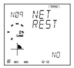
After configuring the AXM-WEB-PUSH module, press the **H** and **V/A** buttons simultaneously, the screen will go blank and **Setting** will be flashing. From here users can press either the **P** or **E** buttons to navigate to **Meter** and then press **V/A** to navigate back to the main metering page.
