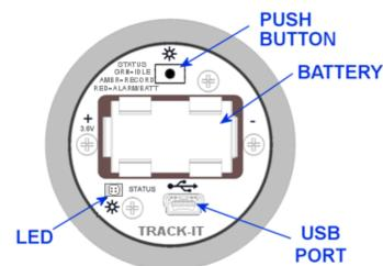
**Serial Communication:** The logger has a mini USB port. Plug the cable into this port and the other end into the USB port on your PC/Laptop. The provided software needs to be installed in order to work with the logger.
