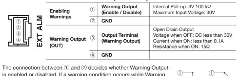
is enabled or disabled. If a warning condition occurs while Warning Output is enabled, a connection between (3) and (4) will be established and a warning will be output.
