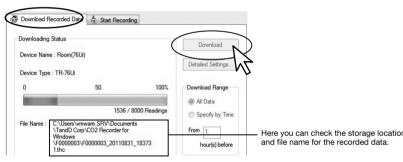
**3.** When a completion message appears after downloading, click the [OK] button to view the graph for that data.
