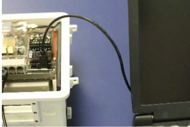
Figure 8: Connecting the U30 to a computer
