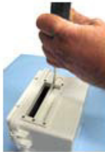
Figure 27: Opening Secondary Cable Slot
