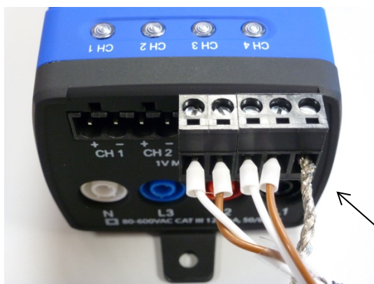
Shield Wires from DENT RoCoil CTs connected to ELITEpro XC
