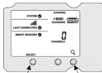
Press the Select button to view the smart sensor channels
