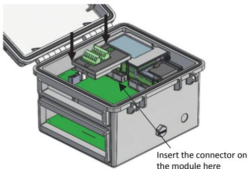
**WARNING:** If you inadvertently install modules while the power is on, you must disconnect and then reconnect the battery and charging device to guarantee proper operation.
