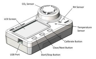
**USB Port:** Use this port to connect the logger to a computer for use with HOBOware or to power the logger for longer deployments or if faster logging intervals are required.
