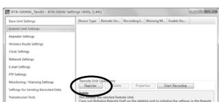
2. When the [Connect a Remote Unit] dialog box appears, unplug the USB cable from the Base Unit (1) and plug it into the Battery Charge Dock\* (2).
