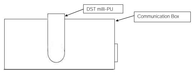
Figure 4.1 Inserting Recorder into the Communication Box
