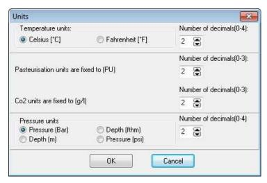
Figure 8.2 Temperature and Pressure Unit Dialog Box
