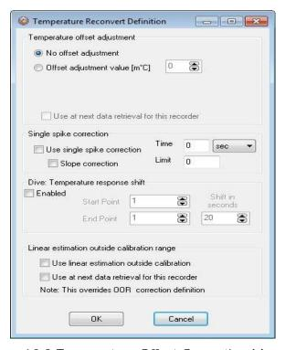
Figure 10.2 Temperature Offset Correction Menu
