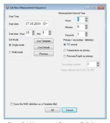
Figure 5.6 Measurement Sequence Definition
