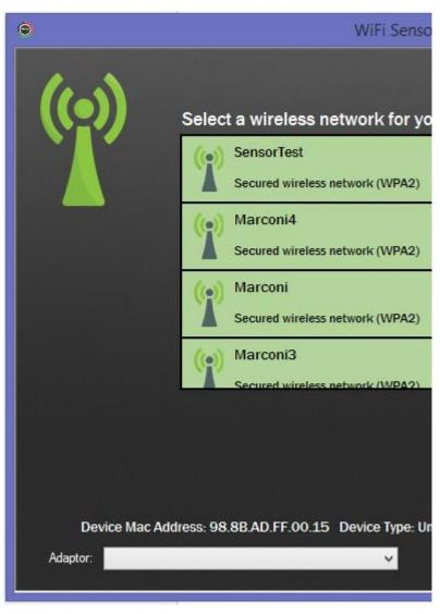
On the Wireless Network selection screen, click on the green antenna symbol on the top left of the window. This will cause a dropdown box to appear on the bottom left. Select the network adaptor which corresponds to the same network as the WiFi Sensors. Then continue the setup as normal.
