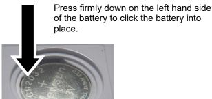
3.2 Replace the battery door; turn clockwise to lock it into place.
