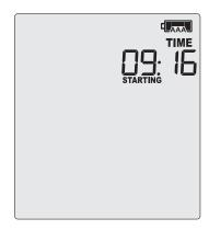
Once **READY** disappears, release the button within two seconds. **STARTING** will now disappear, and the **REC**• symbol will be shown. The UTRED30-16 now records temperature data.
