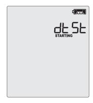
The UTRED30-16 will perform a Connection Test as soon as the recording has started. To check the connection before the start time is reached, you can initiate the connection test yourself. Please refer to Testing your wireless and network connection (on page 1).
