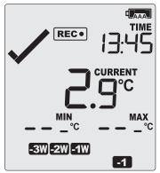
The logger will now track new min/max values. A min/max reset mark will be recorded in the logged data. As soon as the next reading is taken, both minimum and maximum values will be shown again. You will be able to see on the PDF and in the summary in LogTag® Analyzer when the min/max values were cleared, but you will not be able to review previous min/max values on screen once they have been cleared.
