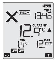
Each alarm trigger condition consists of a threshold temperature value, an activation type (which can be instant, consecutive or accumulative<sup>2</sup>) and a delay time, if it is not an instant alarm.
